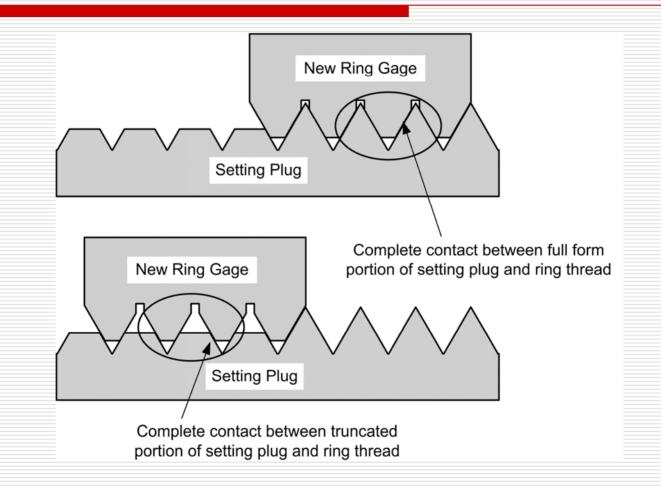
With the ring on the truncated portion of setting plug examine for side-to-side wobble.
